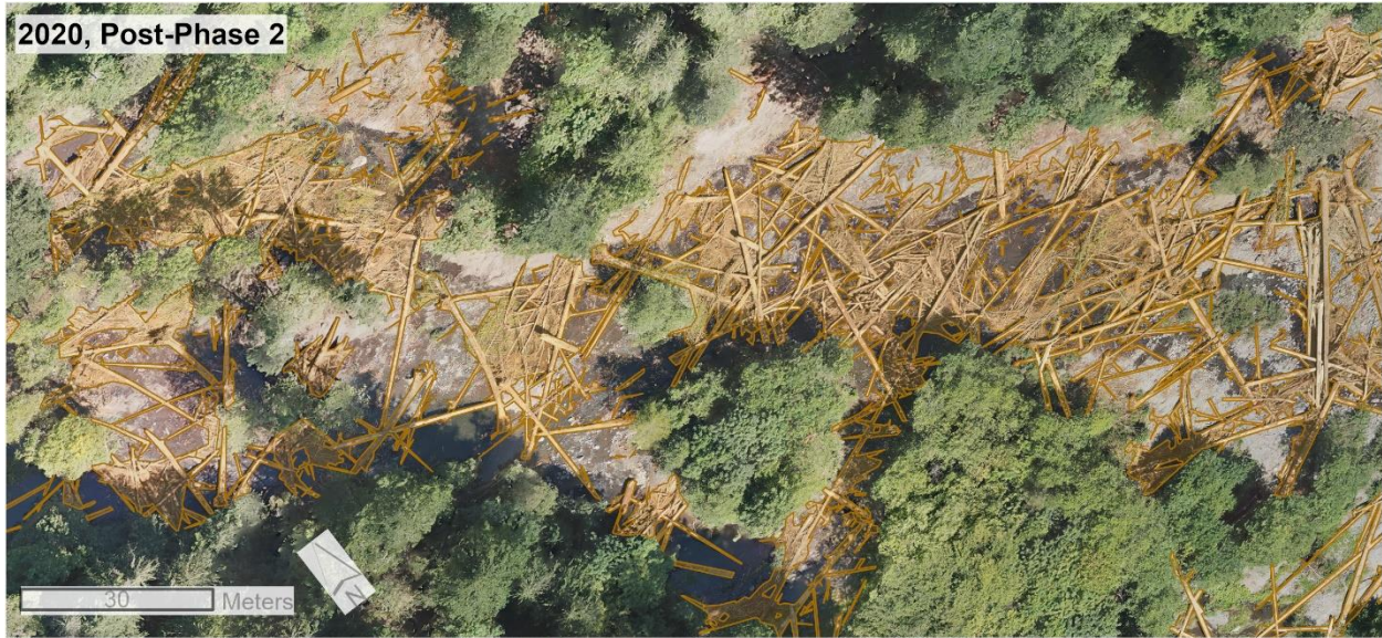
Figure 15: Orthomosaic imagery showing the wood lattice placed as part of phase 2 restoration. Wood is highlighted in brown for clarity.
