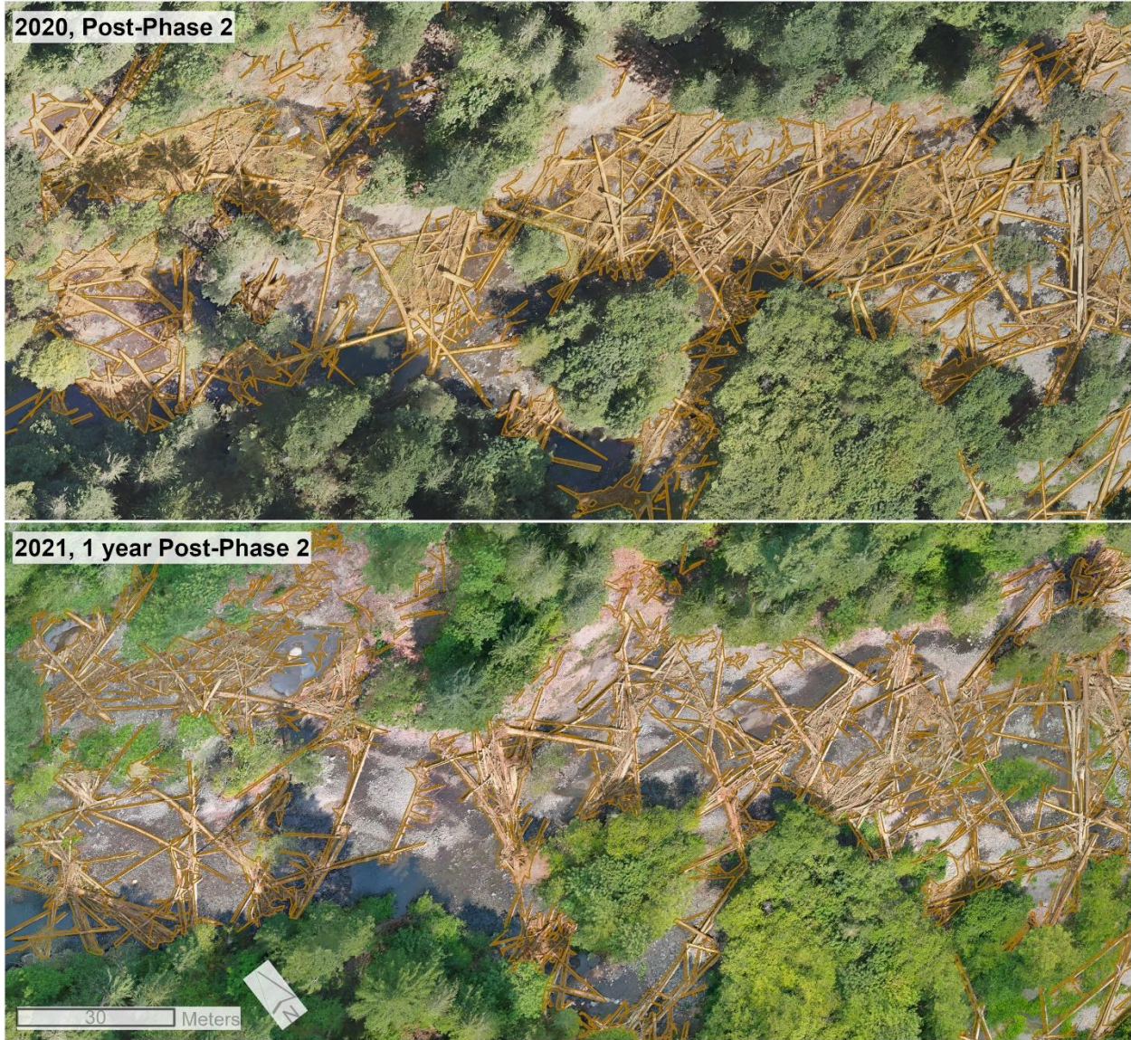
Figure 20: Orthomosaic imagery showing wood rearrangement from just after phase 2 restoration to 1 year after phase 2 restoration. Wood is highlighted in brown for clarity. Note that while both images show a wood lattice, some discrete jams, or denser accumulations of wood, have formed in the lattice in the year following restoration.
